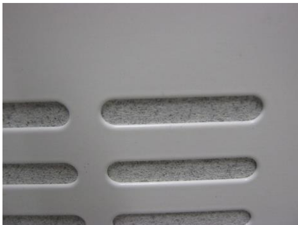
Photo 15: Tested product 200465-1 detail openings in door with acoustic filling
